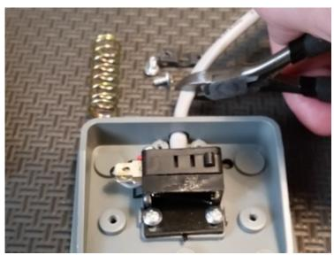
Using wire cutters, cut the cable about 1.5 inches (4 centimeters) past the pedal base.
