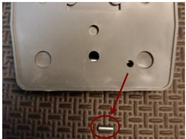
Carefully tip the pedal over and catch the small metal pin. Place it in a safe place with the screws.
