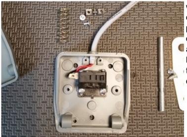
with 2 screws, holding the cable onto the pedal base in the above picture. Using your screwdriver, carefully remove the two screws and the black plastic bracket holding the wire. Do not remove the switch assembly in the center of the base yet.
