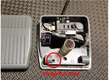
Place the spring on the raised circle on the pedal base. There is also a raised circle on the pedal top that you'll need to mate with while you bunch the halves together to put the hinge pin back in. It is not hard but you have to exercise some care.
