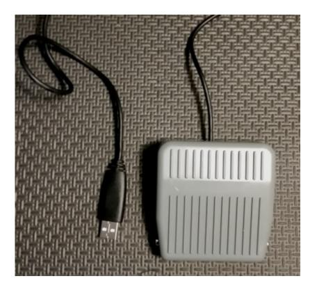
The USB foot switch should work with Windows, Linux, or Mac from the last few years (with plug and play, which has been around for quite a time). When you plug in the USB cord, the computer will detect something is plugged in but it will not know it's the switch until the Trinket boot code finishes timing out in a few seconds. Then your operating system device list will show a keyboard device entitled "Trinket Keyboard".
