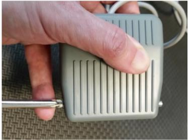
pin. Keep pressure on the pedal (it is spring loaded) while using pressure to push the hinge pin out.
