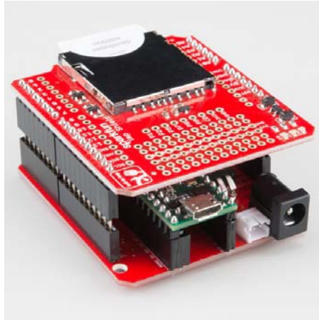
Final Adapter assembly with the Electric Imp Shield stacked on top.
