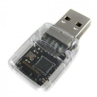
The FLIRC USB dongle allows the use of any remote control with your Raspberry Pi. Configure the device on your desktop PC, then simply plug into your Pi for a perfect media centre companion! Amaze your friends and family when the tiny box stuck to the back of your TV controls your entire media collection using an old DVD remote!
